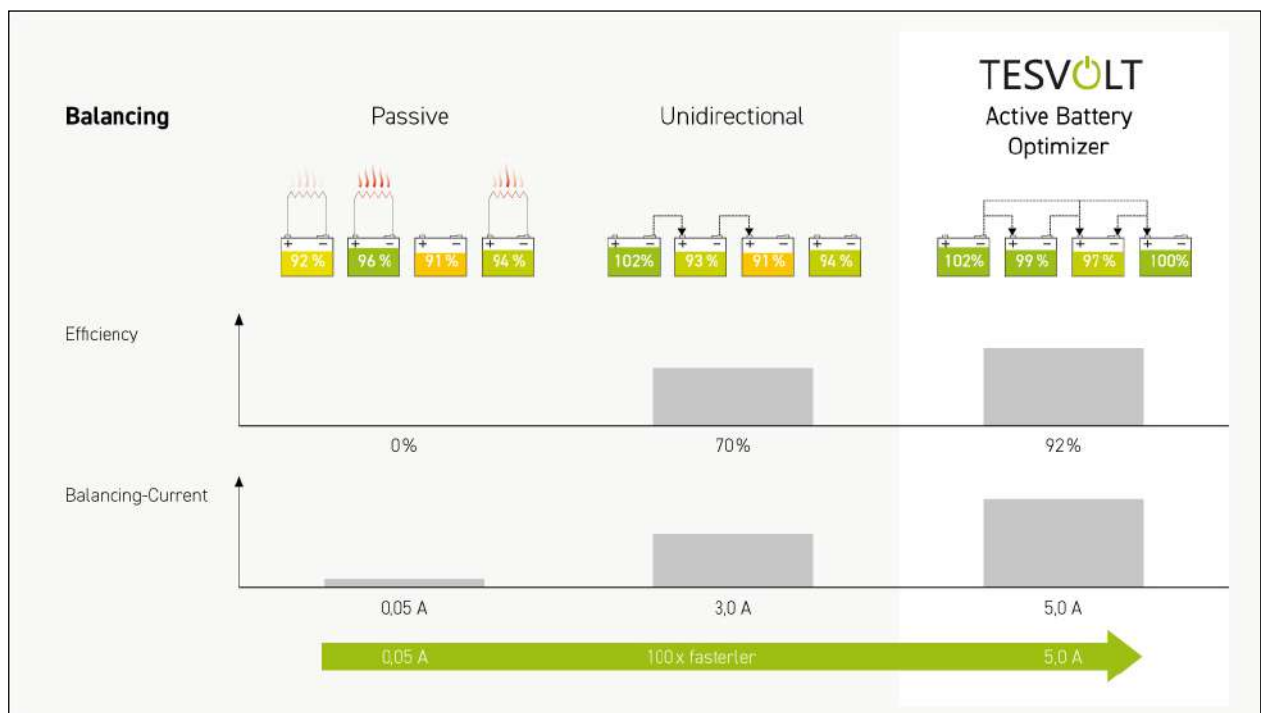
Figure 31: Cell Balancing by Tesvolt
